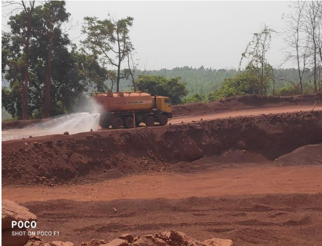
Photo showing water tanker sprinkling on road and dry fog system at screen plant
