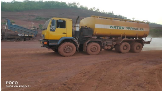
Mobile Water Tanker for dust suppression on mines haul road & Dry fog system at screen plant
