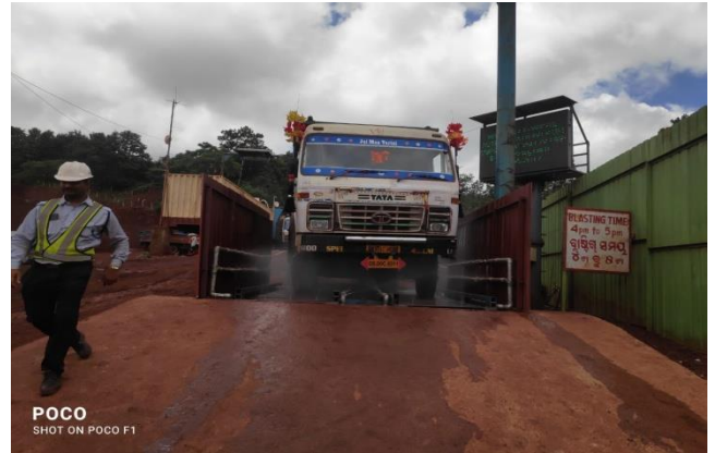
Photo#02: Truck wheel washing system installed at mines main gate
