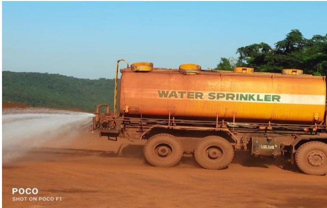
Photo#01: Mobile water Tanker engaged for dust suppression
