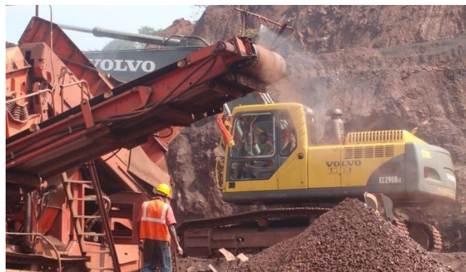
Photo#03: Mineral handling plant with dust suppression arrangement
